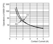
Test conditions: Single contact type: AgNi, Resistive load, 250VAC / 30VDC, Room temp., 1s on 9s off
